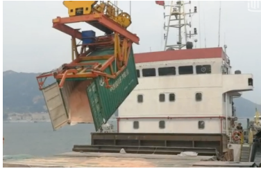
Figure 6 Realistic picture of fully automatic "centralized to scattered" automatic door opening and closing technology operation
