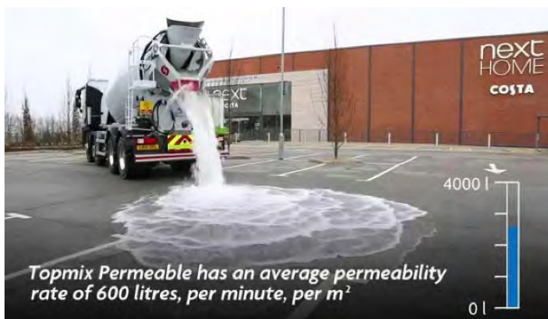
Figure 42. Test of permeability of self-draining concrete [245]
