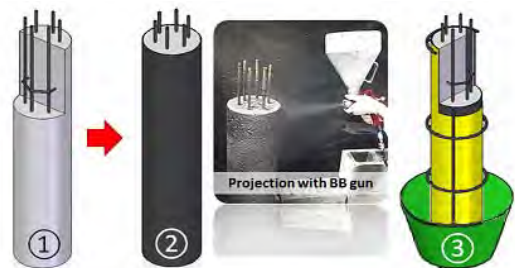
Figure 27. Device assembly with self-sacrificing concrete anode: (1) Self-sacrificing concrete is sprayed by using a compressed air gun on the surface of the specimen. (2) An absorbent layer of polypropylene is placed recovering the specimen surface. (3) The electrical circuit is installed. The positive pole of the source is connected to the anode, and the negative pole is connected to one of the longitudinal of the specimen reinforcement [198]
