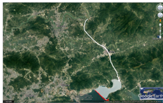
Figure 13. A 45 km canal to divert Dong River to a coastal reservoir which is enclosed by 10 km seawall, 40 km 2 surface area, about 60 km to Shenzhen and Hong Kong.
